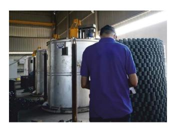
Due to the repeating hammering or other work in the first basic forging process, the metal's ductility is reduced to some extent. Thus, to restore metal's ductility to the fullest, the Annealing Process is done by our automated temperature control system which helps to stable the toughness of bearing with reduced hardness and strength. This is because, if the material becomes too hard, it can make working nearly impossible or results in cracking.
